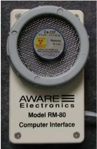
Fig. 3 – HotBits Geiger-Müller tube interfaced to a computer's serial I/O port
